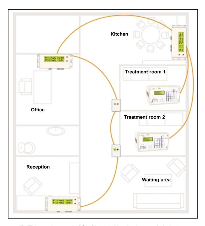
The FTI-1 has a network connector (RS-422) that outputs information about the running treatment program to monitoring LCD displays that can be placed anywhere within 300meters (1000ft) of the FTI-1
